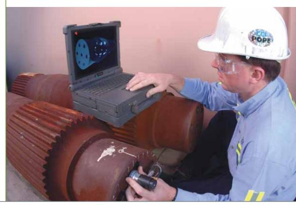
A CCI Pope technician verifies the presence of spline cracking detected by ShafTest™ in the final drive shafts of a mining shovel.
