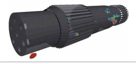
This 3D model – the output of ShafTest™ – confirms the presence of spline cracking defects (multi-coloured patches) in the final drive shafts of a mining shovel.
