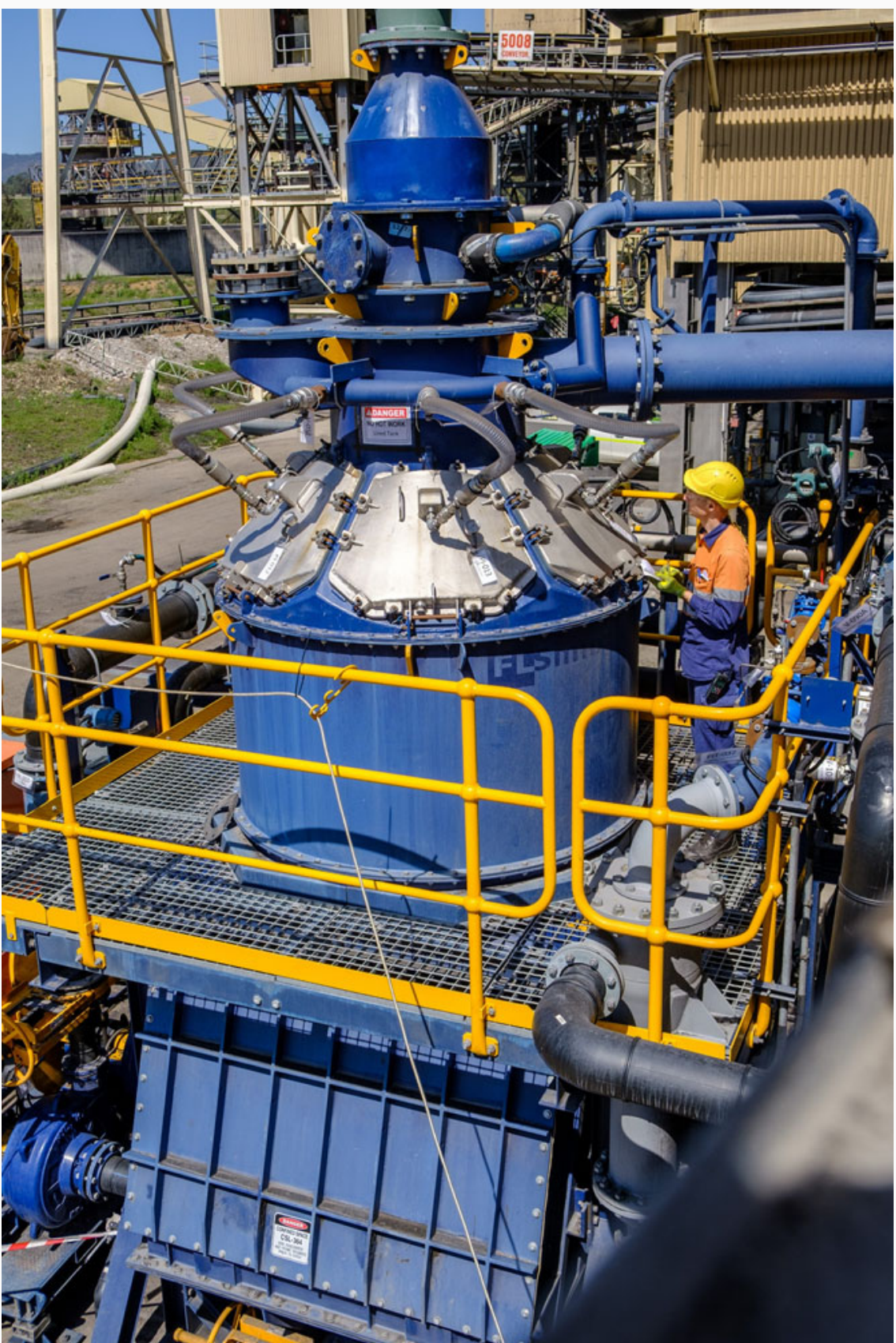
The Reflux Flotation Cell (photo courtesy FLSmidth). FLSmidth has an R&D agreement with the University of Newcastle and an exclusive licence agreement to manufacture, supply and support the technology. FLSmidth has also been providing considerable support for the trial. Other key inputs have come from the
