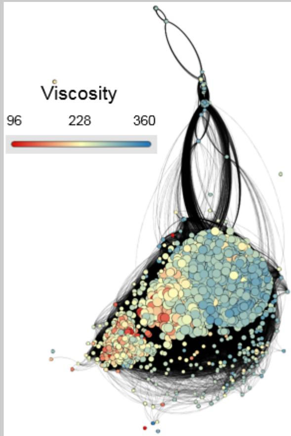
Figure B - Graph coloured to reflect range of viscosities. Includes all left final drive samples. A quick review of the graph shows that low viscosity is a clear issue for the dozer final drives.
